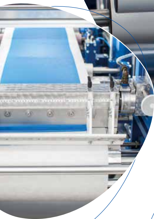
Coating head with optional viscosity measurement
