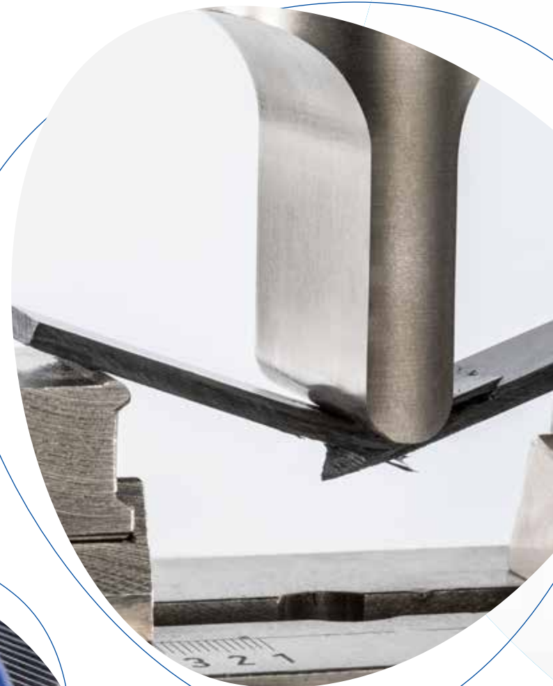
Carbon fiber composite bending test
