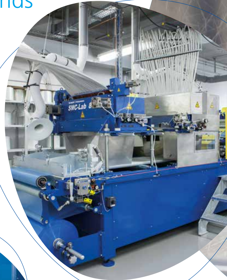
SMC line with glass and carbon fiber cutting system
