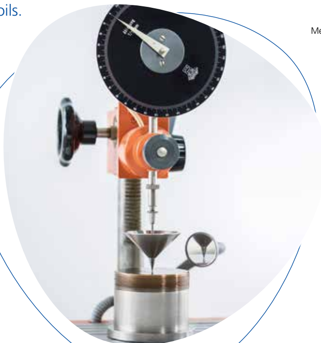
Consistency measurement with a penetrometer
